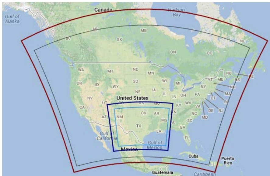
Figure 9. WRF modeling domains at 36-km grid spacing (red) and 12-km spacing (dark blue), and corresponding CAMx domains at 36-km spacing (gray) and 12-km spacing (light blue). http://www.tceq.texas.gov/airquality/airmod/rider8/modeling/domain .
